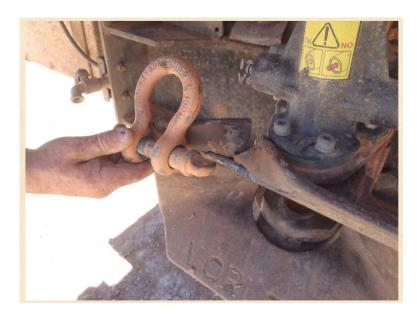
Recently a DEWNR employee attempted to recover a bogged contractor vehicle using two snatch straps joined with a shackle. The weight of vehicles involved (a DEWNR 4WD truck and the contractor's semi-trailer) exceeded the rated capacity for the snatch straps and as a result a strap broke and the shackle recoiled into the DEWNR vehicle breaking the towing hitch.
