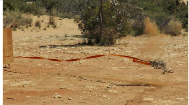
Photo show a chain attached about 2m from the end of the snatch strap using the Prusik knot
