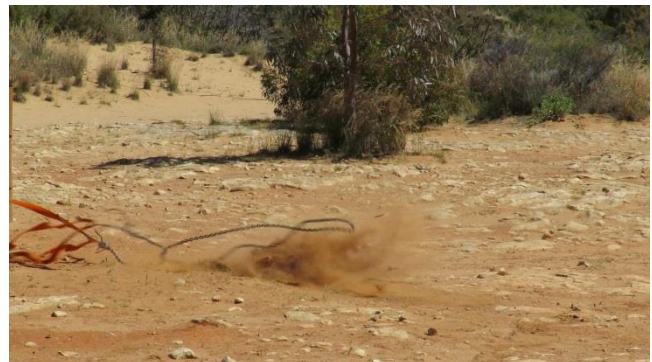
Attached end of 1 chain about 3m from each end of snatch strap – the camera doesn't show it, but the whole chain hit the board
