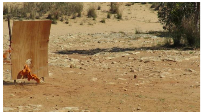
The next frame (1/30th of a second later) The shackle punches a big hole in the plywood. The shackle ended up about 10m further on from this picture
